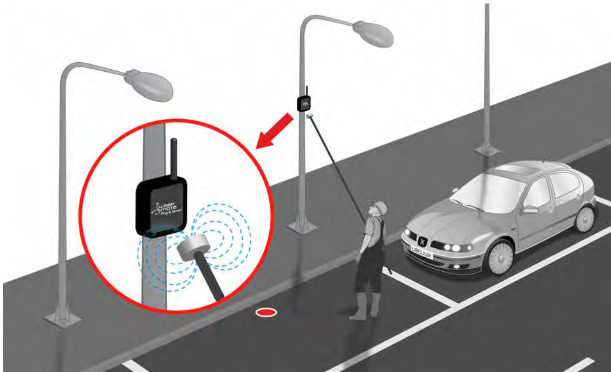
Figure: Resetting a Plug & Sense! node with a pole and magnet
