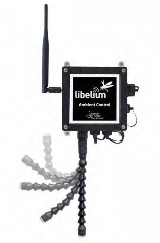
Figure: Configurations of the Luminosity sensor probe (luxes accuracy)
