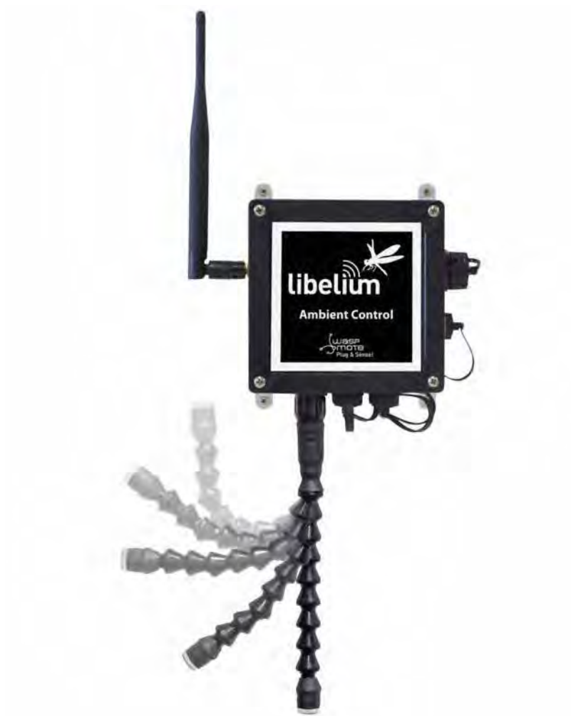
Figure: Configurations of directionable sensor probes
