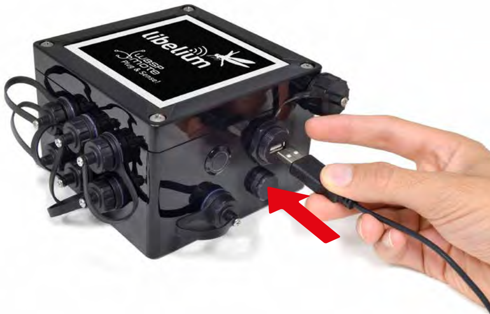
Figure: Connecting the USB cable to Wasmote Plug & Sense!
