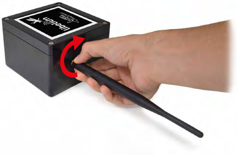
Figure: Connecting antenna to the enclosure
