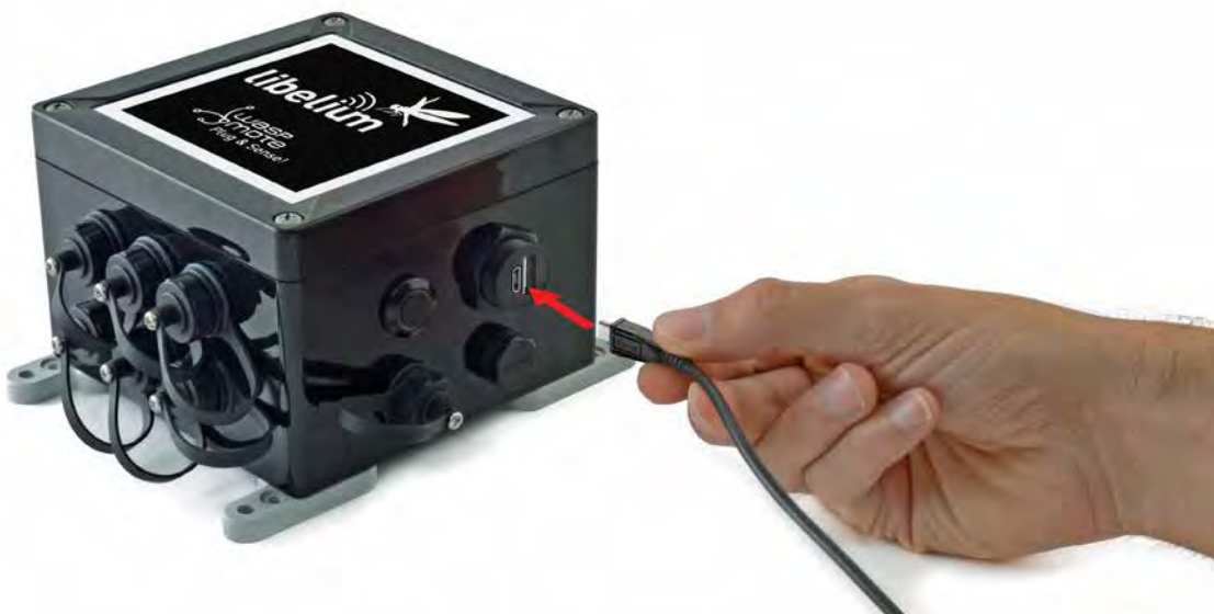
Figure: Connecting the micro-USB cable to Plug & Sense!
