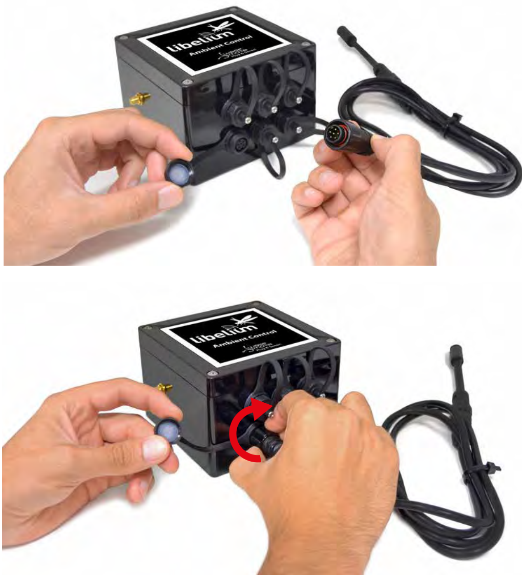
Figure: Connecting an extension cord to the enclosure
