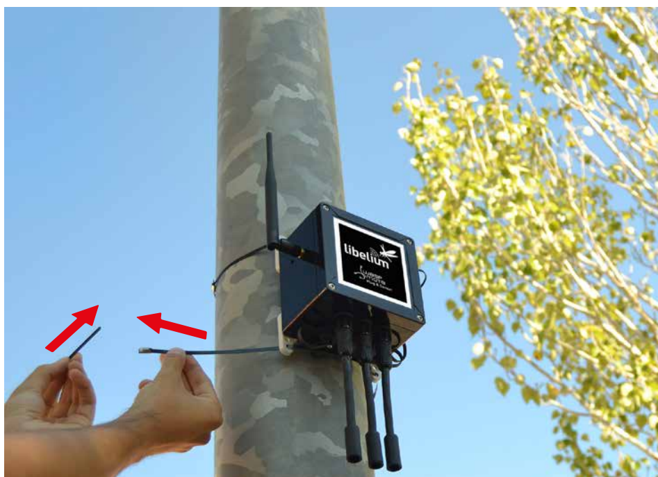
Figure: Placing Wasp mote Plug & Sense! on a street light
