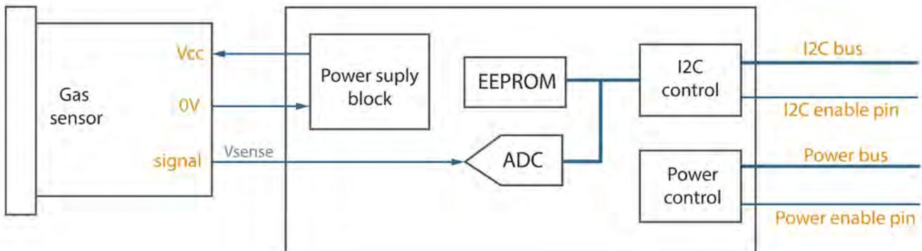
Figure: NDIR AFE module diagram block
