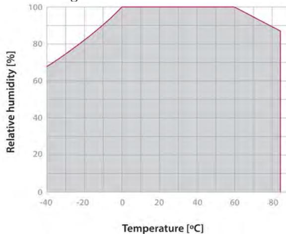
Figure: Humidity sensor operating range
