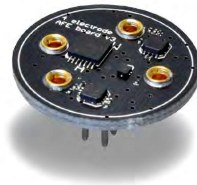
Figure: 4-electrode AFE board
