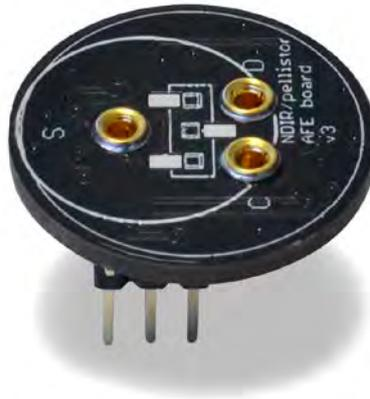
Figure: AFE board for pellistor and NDIR
