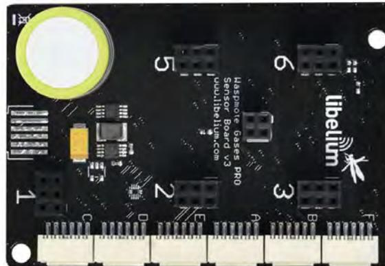
Figure: Image of socket 4 with a 3-electrode sensor
