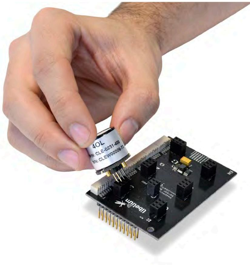
Figure: Connection of a 3-electrode AFE board
