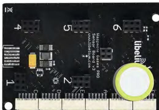
Figure: Image of socket 3 with a 4-electrode sensor
