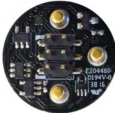
Figure: Bottom view of a 3-electrode AFE board
