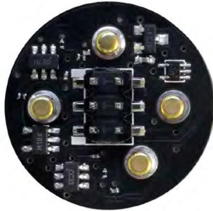
Figure: Bottom view of a 4-electrode AFE board
