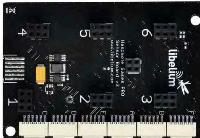
Figure: Top side of the Gases PRO Sensor Board
