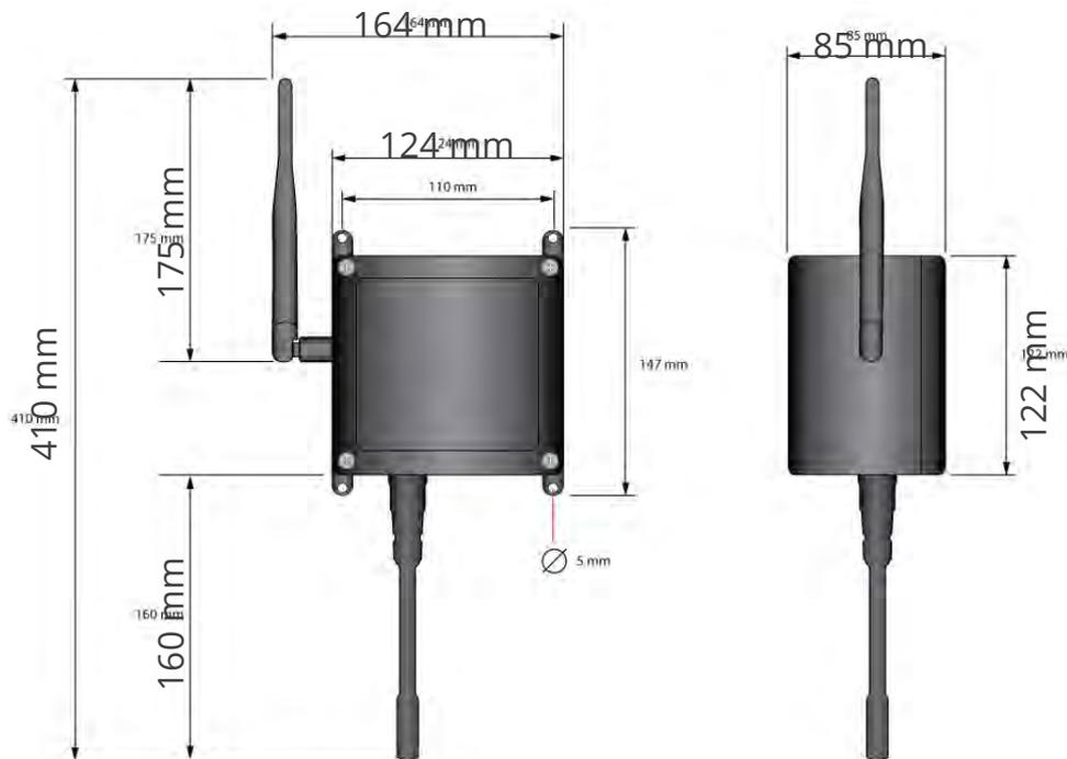
Figure: Main view of Wasmote Plug & Sense!
