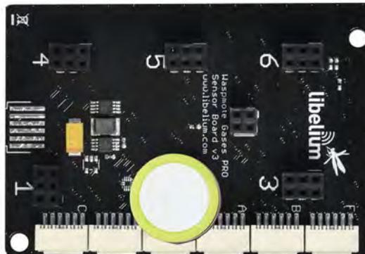
Figure: Image of socket 2 with a 3-electrode sensor
