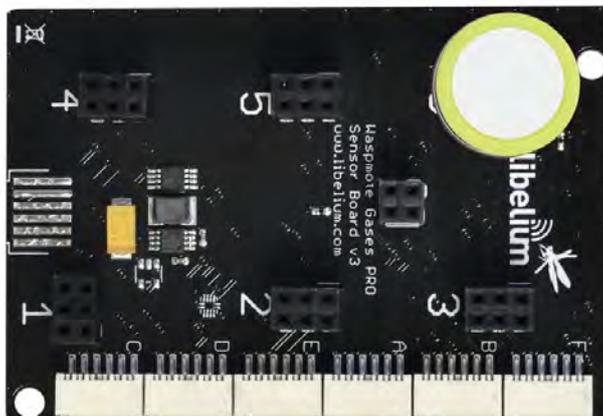
Figure: Image of socket 6 with a 4-electrode sensor
