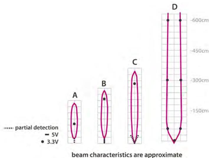
Figure: Diagram of the sensor beam extracted from the data sheet of the XL-MaxSonar®-WRA1™ sensor from MaxBotix
