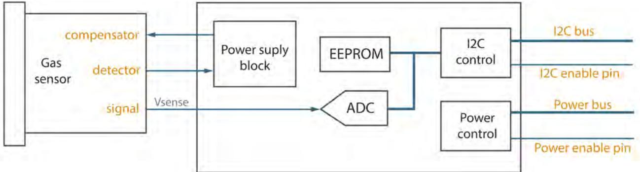
Figure: CH<sub>4</sub> and Combustible Gases Sensor AFE module diagram block
