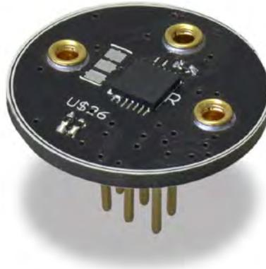
Figure: 3-electrode AFE board
