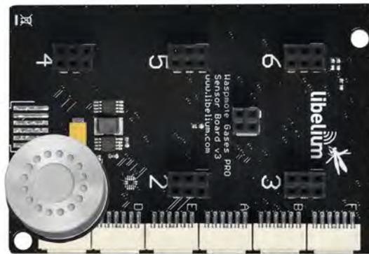
Figure: Image of socket 1 with a 3-electrode sensor
