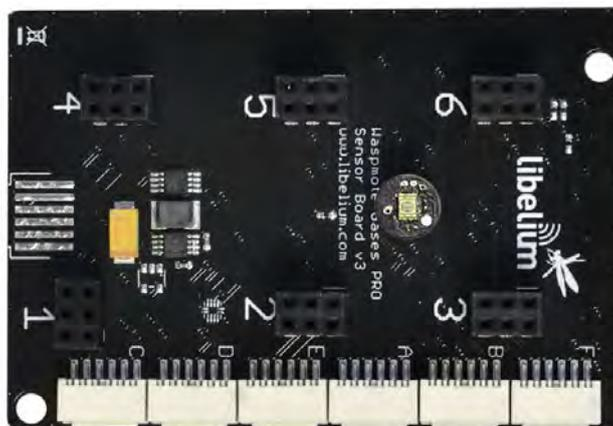
Figure: Image of the socket for the luxes sensor
