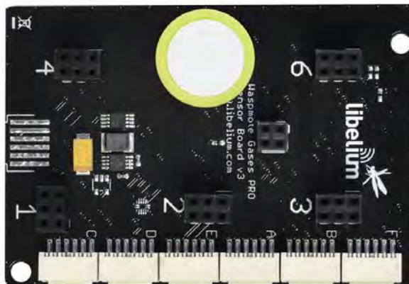
Figure: Image of socket 5 with a 3-electrode sensor
