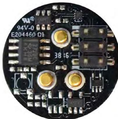
Figure: Bottom view of a pellistor/NDIR AFE board
