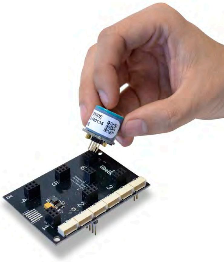
Figure: Connection of a 4-electrode AFE board
